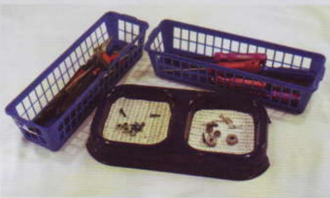
Inexpensive plastic pet food dishes and miscellaneous baskets are cheap accessories for a portable workspace. I spent $2.25 on these. Put a piece of non-slip shelf liner inside the dish to limit the movement of small parts.
